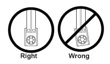
When tightening the screws, be sure to keep bracket parallel to the rail. Otherwise, the rail may bow when opener is operated.
